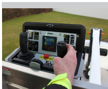
Automatic outrigger setup and packing
